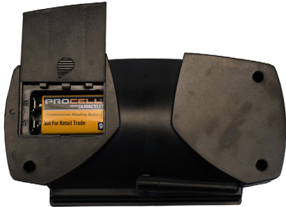
9 volt battery back up is recommended for DROP Hub.
